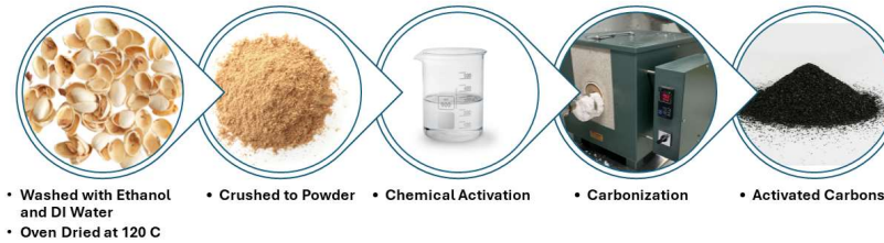
Fig. 2. Schematic of the preparation of AC using NaCl as activating agents.
